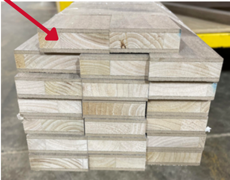
Solid poplar core cabinet panels w/ CNC routed openings
